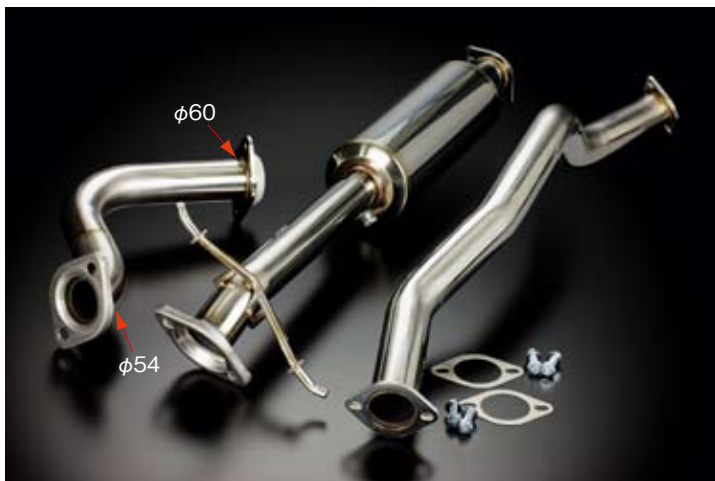
SWIFT SPORT ZC31S/M16A Φ60mm with Circuit Catalyzer 18000-ZC3-10F Price 116,000 yen
